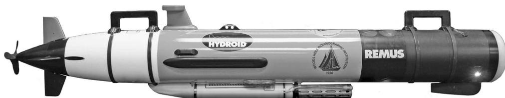
Fig. 2. The customized autonomous underwater vehicle REMUS. Vehicle length is approximately 1.8 m. The vehicle is capable of reaching depths of 90 m. Note the SeaBird 49 CTD attached to the lower portion of the vehicle and the excitation light of the BB2F fluorescence meter.
